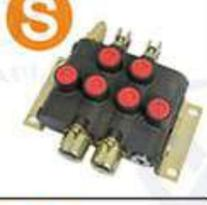
ZS-L20 Series                       | E:16Mpa<br>F:20Mpa<br>G:25Mpa<br>H:31.5Mpa | 100          | 1-15      | O,A,Y,Q        | T:Spring Return<br>W:Detent Control | M<br>G<br>UNF<br>NPT |                                                       |
