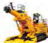
Excavation Machinery / Road Header
